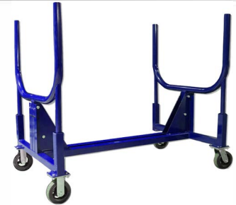
Rolling Cradle (ME-68U) - The rolling pipe cradle is specifically designed to transport large bundles of conduit, pvc and copper pipe, small bore steel pipe and threaded rod in one large cradle. Dimensions- 56"Lx34"Wx34"H. Capacity: 1,000 lbs.
